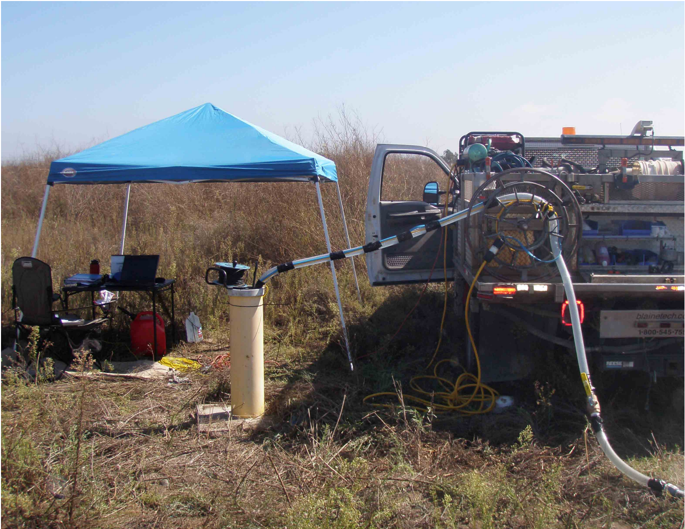
Grundfos 4" Submersible Pump, In-Situ miniTROLL Pressure Transducer, Trailer-Mounted Diesel Generator & Halogen Lighting
