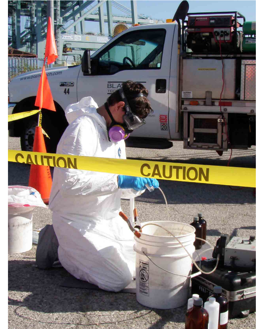
Discrete Sampling Below SPH / LNAPL Layer Geotech Peristaltic Pump, YSI 550 DO Meter & Myron L Ultrameter II
