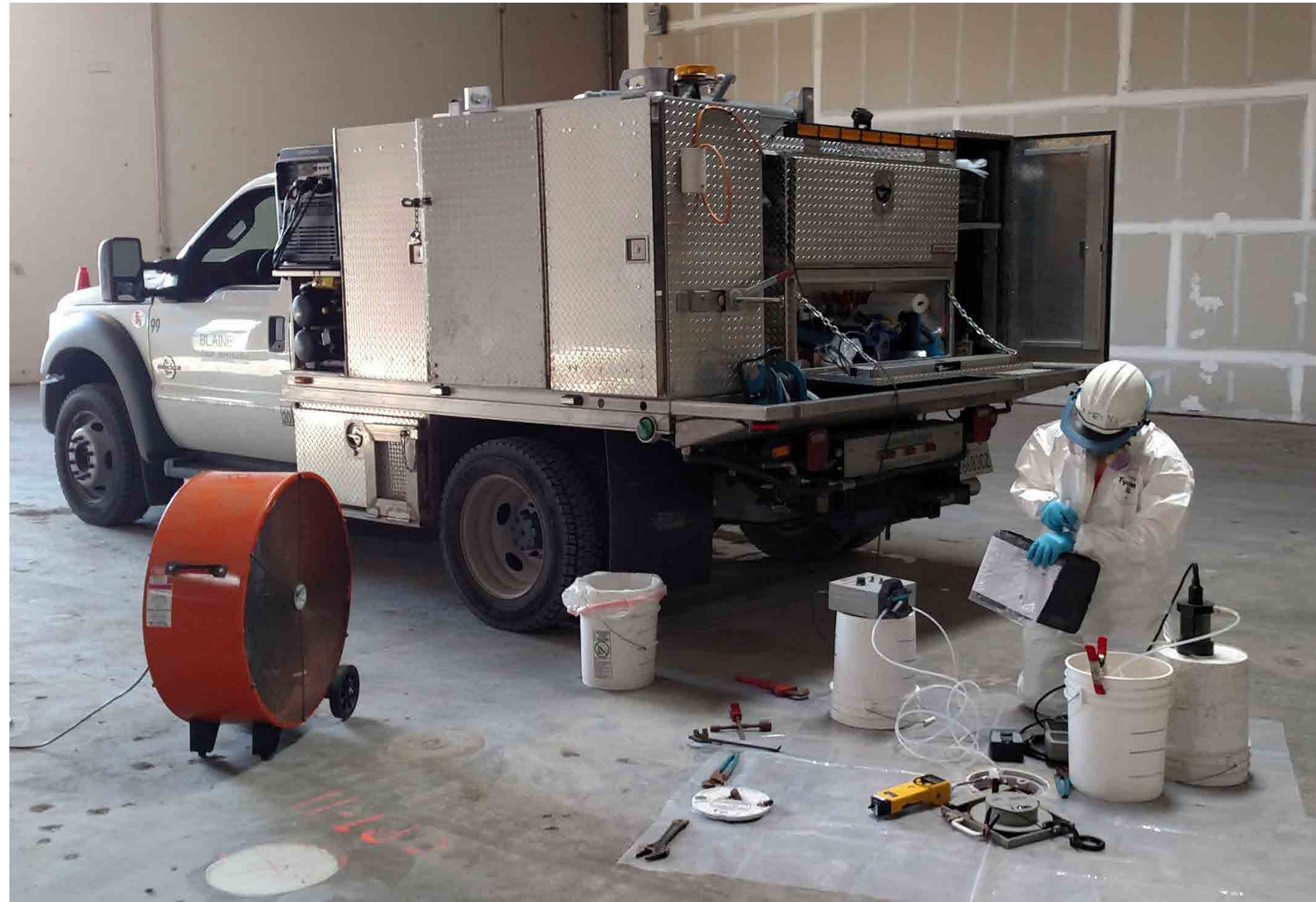
Low Flow Sampling in DNAPL impacted well with Peristaltic Pump, Disposable Tubing YSI Professional Plus Multiparameter Meter & Flow Cell, MiniRAE 3000 PID, Ventilation Fan
